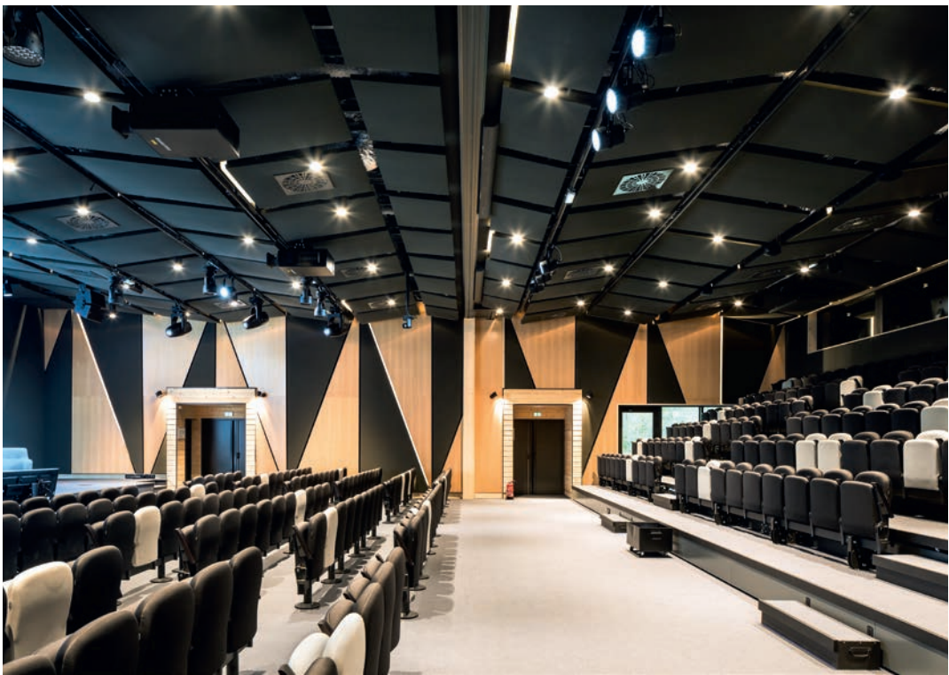
Alternating Stereo panels and reflective panels with Aeria covers on the ceiling. Stretch-fitted Vibrasto cladding on the walls in the same colours. Pernod Ricard University, Domaine de la Voisine, Clairefontaine-en-Yvelines. Cyril Durand-Béhar Architects, Impact Acoustic, 2016.
